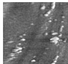
Fig. 4. AFM image (phase contrast mode) of the surface of a silicon-supported PTFE coating etched in a glow discharge plasma.
