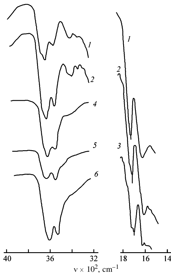
Fragments of the IR spectra of the acetonitrile electrolyte. ( \nu ) Wave number. (1) Initial solution (sample 1), (2) after electrolysis for 15 min (sample 2), (3) after electrolysis for 30 min (sample 3), (4) subtraction of the spectrum of sample 1 (reference channel) from that of sample 2, (5) subtraction of the spectrum of sample 2 (reference channel) from that of sample 3, and (6) subtraction of the spectrum of sample 1 (reference channel) from that of sample 3.
